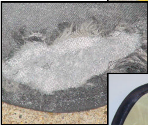
Close-up showing first layer penetration
