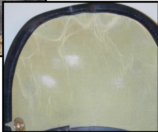
Close-up of backside showing no penetration
