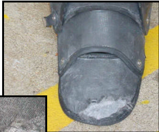
TurtleSkin WaterArmor gaiter accidentally hit at 2500 bar
